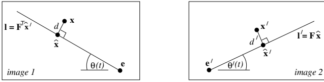
Figure 1: Illustration of Epipolar Geometry. Courtesy R. I. Hartley [4]
