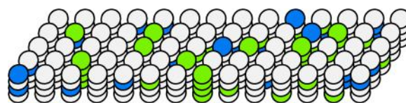
Figure 2.24: Visualization of the TM and the three states. Active in green, predictive in blue, and inactive in white.
