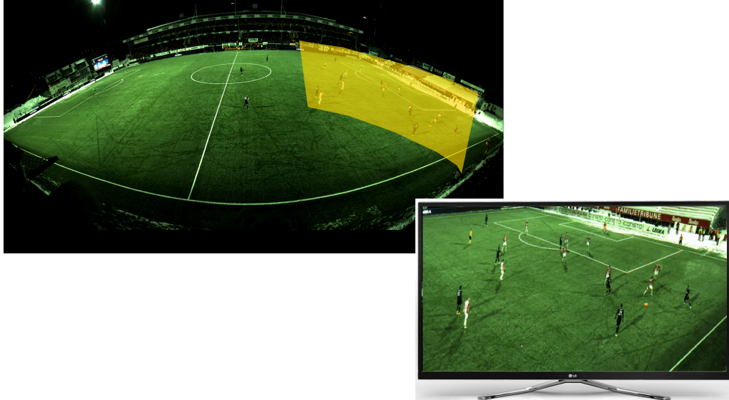
Figure 1.3: The panorama video with the marked region of interest is shown together with the generated virtual camera, emphasizing that the extracted area is not a simple crop from the high-resolution panorama video. It is generated by a perspective re-projection and hence we cannot achieve it by a simple rectangular cropping.
