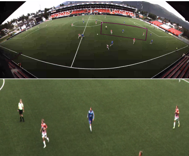
Fig. 6: Reconstructed panorama from multi-quality tiles and the corresponding virtual view. The poor quality in some areas of panorama does not affect the quality of the virtual view.
