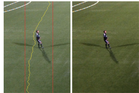
(d) Dynamic stitch with color correction. In the left image, one can see the seam search area between the red lines and the seam in yellow. In the right image, one cannot see the seam, and there are no color differences.
