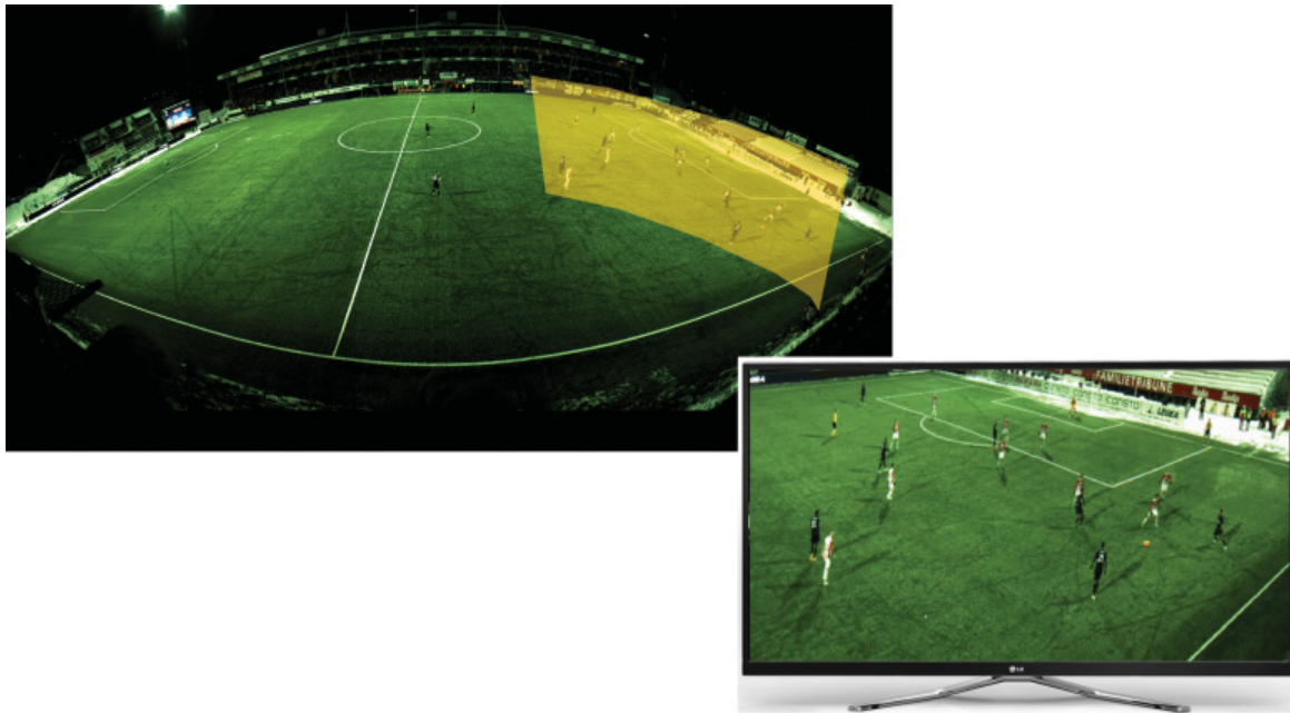
Fig. 2. Virtual view generated from re-projection. The panorama video with the marked region of interest is shown together with the generated virtual camera, emphasizing that the extracted area is not a simple crop from the high-resolution panorama video.
