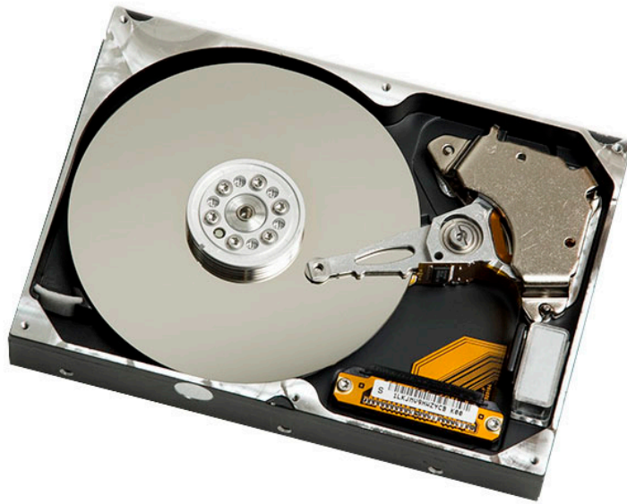
Figure 3.1: Internal view of a magnetic disk [10]
