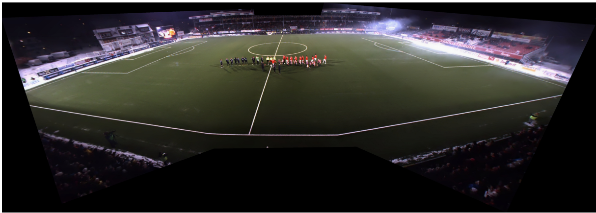
Figure 4.3: An image panorama create with OpenCV's autostitcher, using planar projection
