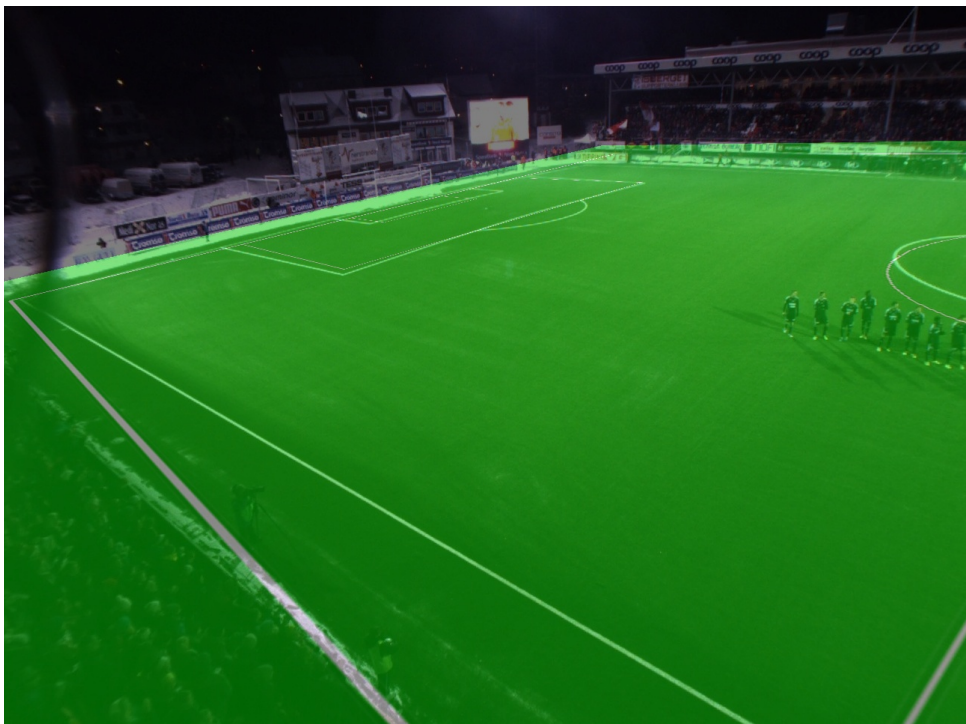
Figure 3.19: Our first attempt to find the homography between the ZXY coordinate plane and the image plane for camera one. The ZXY plane has been warped and superimposed onto the image plane using a miscalculated homography.
