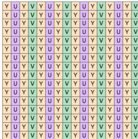
Figure 2.5: Illustration of the memory alignment in a packed YUV image.
