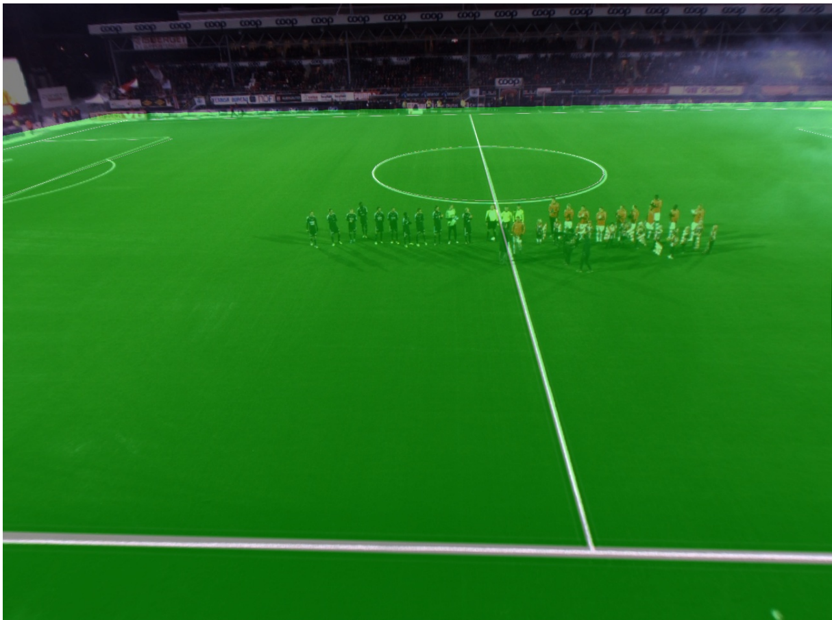
Figure 3.12: The ZXY plane, warped and superimposed onto the plane of the 2nd camera.
