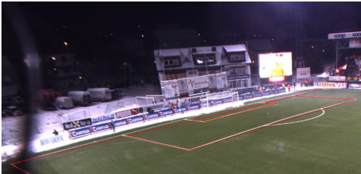
Figure 2.17: The image shows a debarreled image where red straight lines are drawn to illustrate that there is still some barrel distortion in the image.
