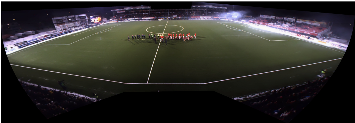
Figure 4.4: An image panorama create with OpenCV's autostitcher, using cylindrical projection
