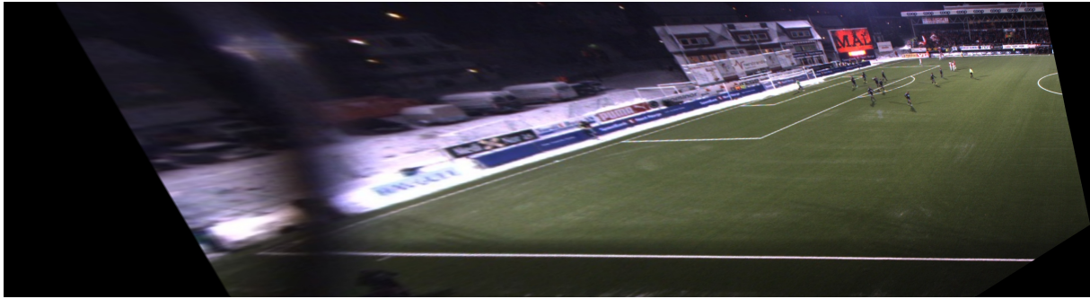
Figure 4.9: The first camera is warped to fit the plane of the second camera with padding calculated. Note that the image is cropped for display purposes.
