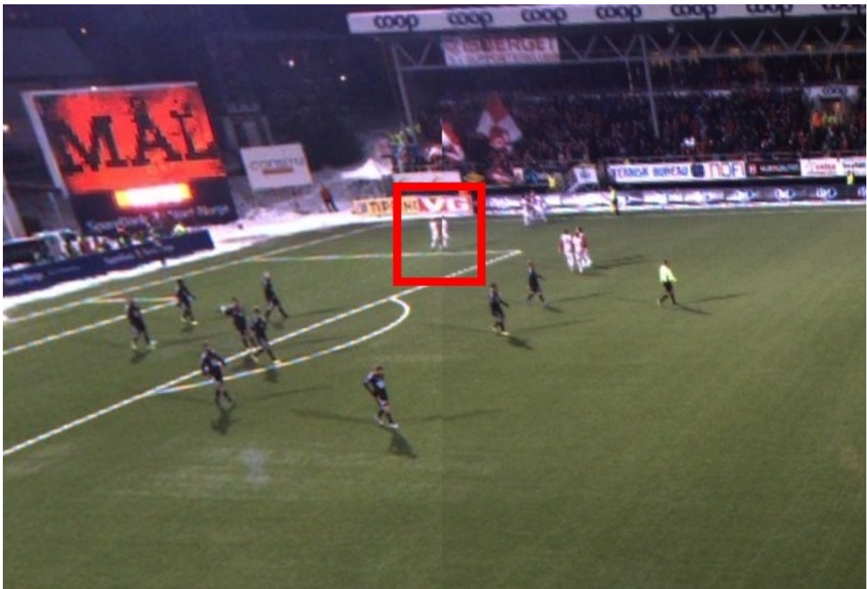
Figure 4.15: An image showing parallax errors where a player appear on both sides of the seam.
