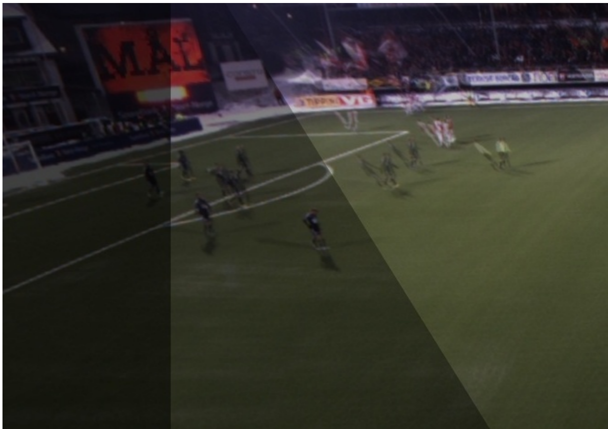
Figure 4.16: An area where three of the cameras overlap which illustrates parallax errors. The most highlighted area is composed of three images superimposed onto each other, the middle one consists of two, while the dark one consist of only one.
