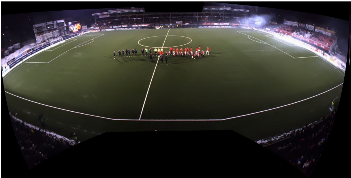
Figure 4.5: An image panorama create with OpenCV's autostitcher, using spherical projection
