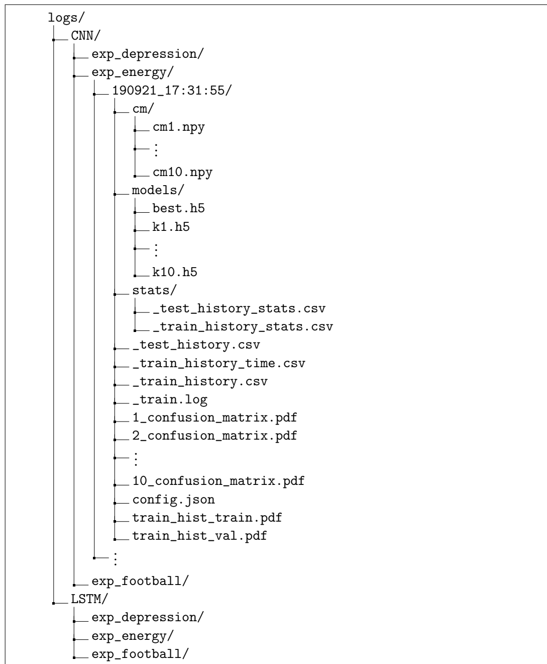
Figure 3.5: General tree structure of stored results and generated logs from the experiment- and evaluation pipeline in our experiment framework. Confusion matrices are stored, accordingly with their respective heatmaps. Our evaluation pipeline also saves the models, best models, history statistics, history, configuration file and history figures.
