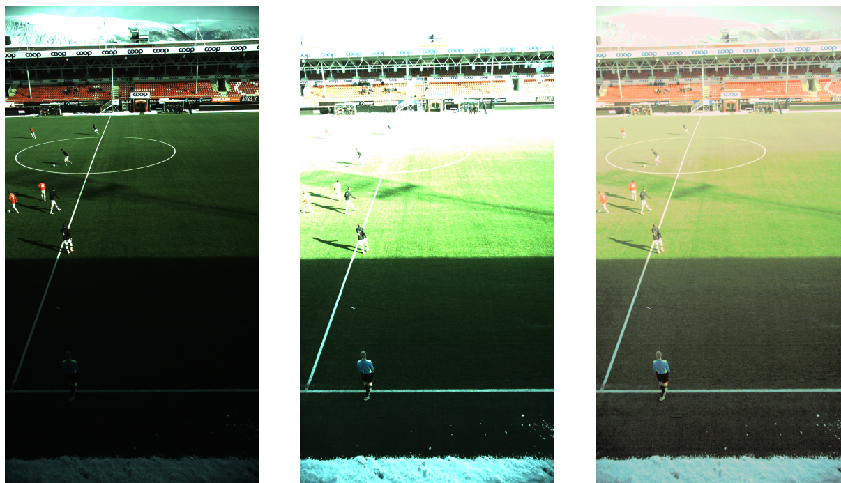
Figure 2.5: Images illustrating the effect of running the pipeline images through the HDR module. The leftmost image (low) is combined with the middle image (high) to produce the rightmost image.
