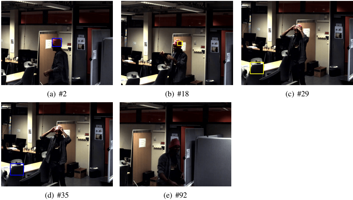
Figure 4.4: The rectangle marks the TLD tracking. Yellow and blue rectangle represent low and high confidence, respectively.
