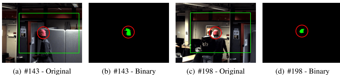
Figure 4.10: An example where strong color results in a much larger binary blob
