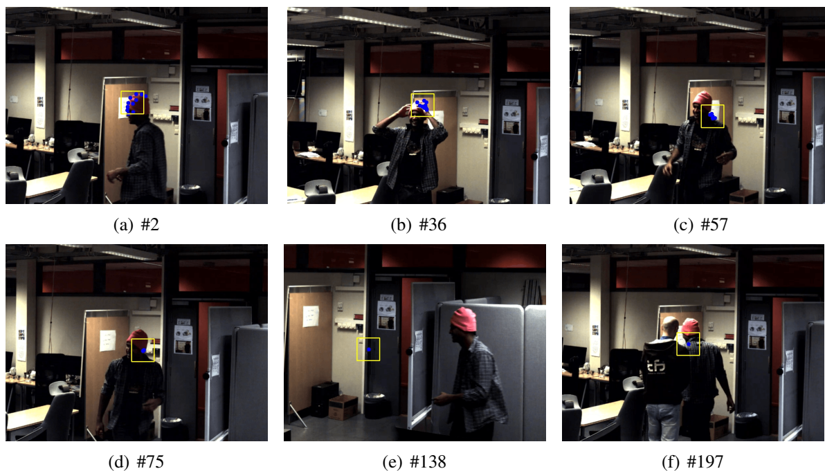
Figure 4.12: The yellow rectangle marks the search area, and the blue dots represent the features found in the area.
