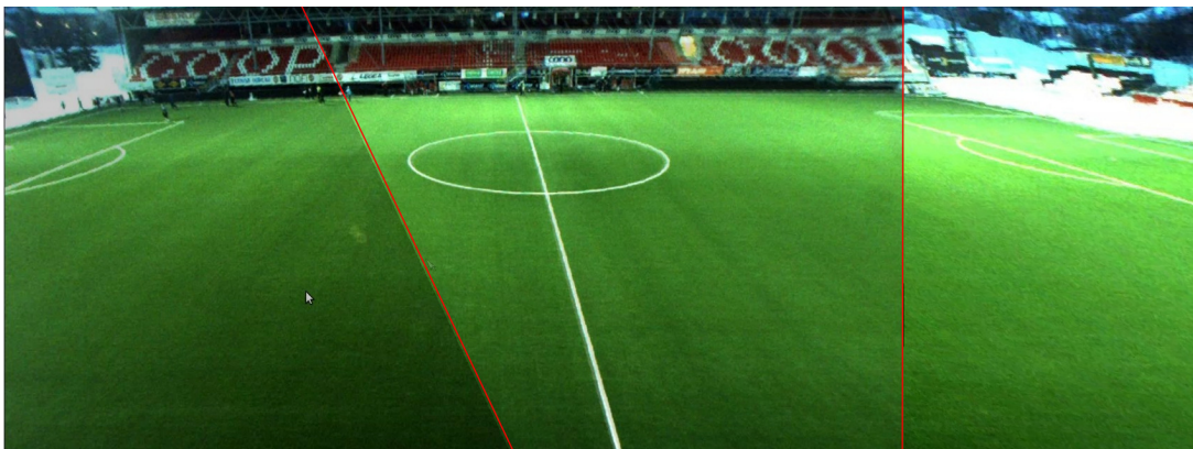
Figure 4.6: Overlapping regions between warped images from camera two and three in the pipeline.
