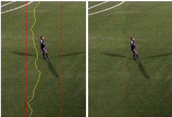
(c) Dynamic stitch with no color correction. In the left image, one can see the seam search area between the red lines, and the seam in yellow. In the right image, one clearly see the seam, going outside the player, but there are still color differences.
