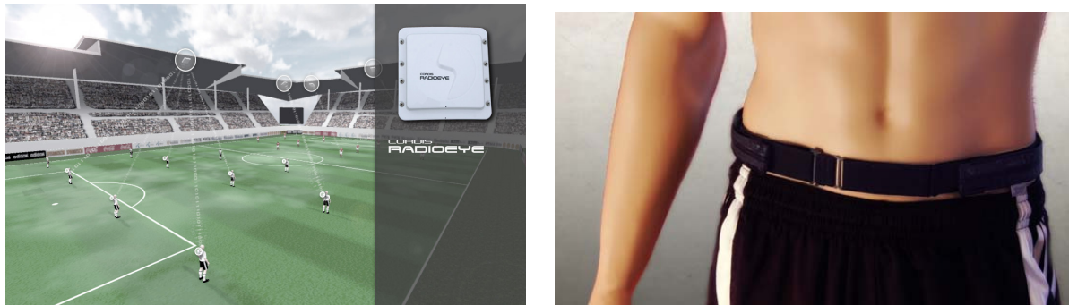
(a) The radio antennas located on the stadiums where the system is implemented. (b) The belt worn by the players. Transmits signal to the radio antennas.
