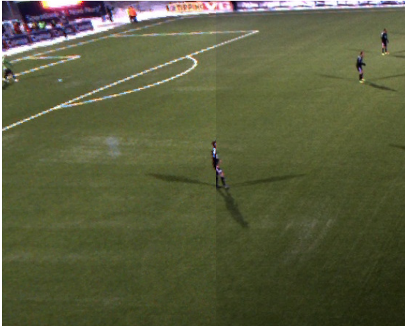
(a) The original stitch pipeline in [24] and [23]: a fixed cut stitch with a straight vertical seam, i.e., showing a player getting distorted in the seam.
