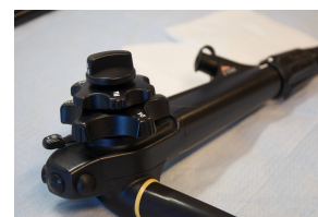
(d) The control unit of the endoscope the gastroenterologist uses to control the endoscope in terms of zoom, rotation, etc.
