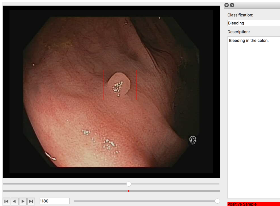
Figure 3.2: The interface of the semi-supervised annotation tool. The user has only to mark the area with the disease and enter the name and a short description of it. The tool then automatically tracks the marked area and stores the examples in a training dataset.
