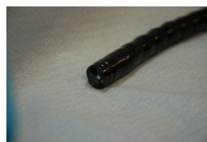
(c) The tip of the endoscope. It is very flexible and can be moved by the gastroenterologist in every possible direction.
