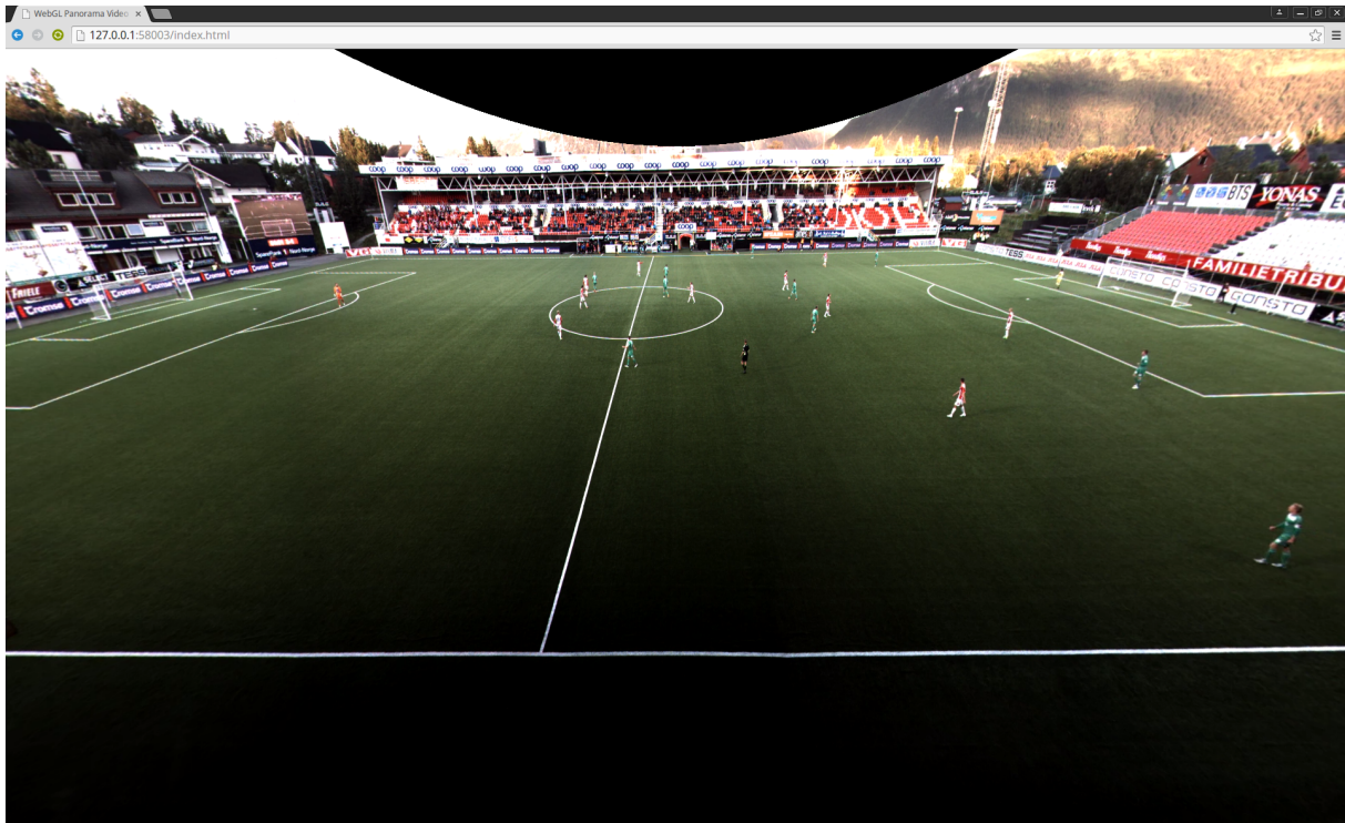
Figure 4.3: Unwarped panoramic video displayed in browser using WebGL-based panoramic video viewer
