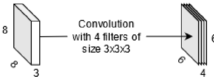
Figure 2.4: Convolution for input size 3x8x8 with 4 filters of size 3x3x3, resulting in 4 feature maps of size 6x6.
