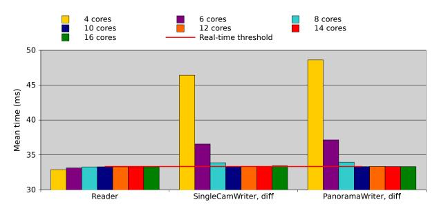
Figure 4.22: CPU core count scalability, write difference times
