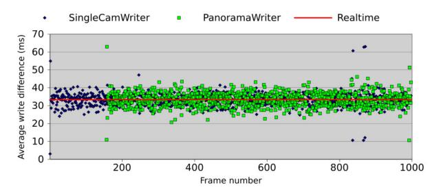
Figure 4.18: Pipeline write differences, 1000 frames run Note that the delayed start of panorama writes is caused by the frame delay buffer described in section 4.4.4
