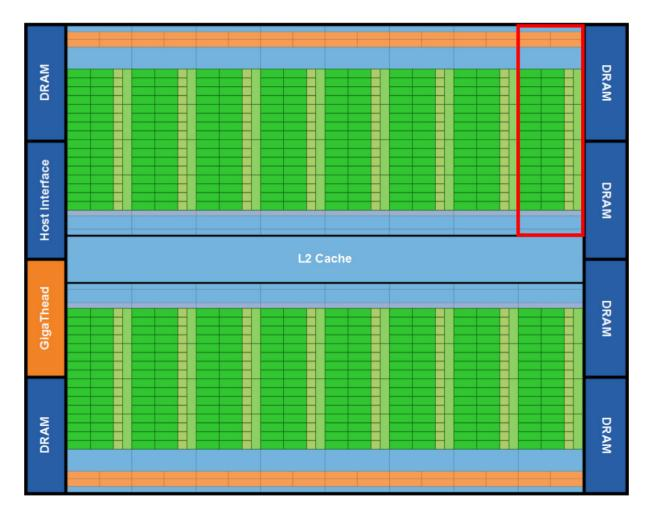
Figure 3.1: The Fermi architecture [3] An example Stream Multiprocessor (SM) marked in red.
