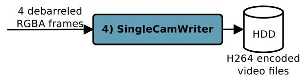
Figure 4.6: The SingleCamWriter module
