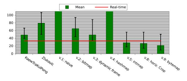
Figure 5.7: Performance of CPU based ZXY BGS implementations, camera 2 (ms) Note that the lookup- and calculation-based cropping versions are excluded, because they were tested on camera 1.
