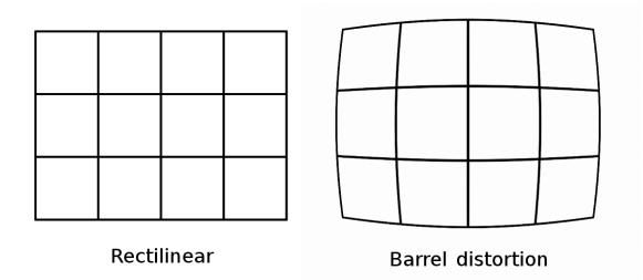
Figure 2.6: Original and rectilinear image vs. barrel distorted version [2]
