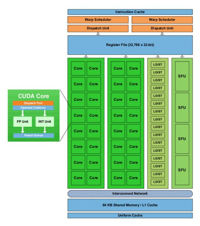
Figure 3.2: A Fermi Stream Multiprocessor [3]
