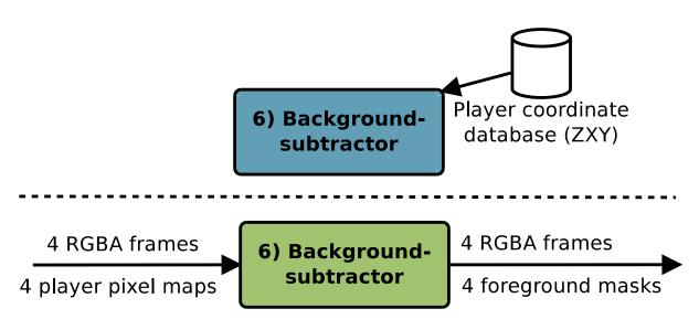
Figure 4.8: The BackgroundSubtractor module
