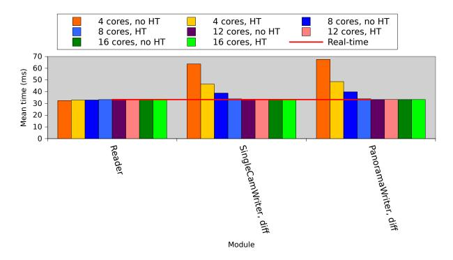
Figure 4.24: HyperThreading scalability, write difference times
