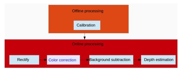
Figure 5.13: The depth map calculation pipeline
