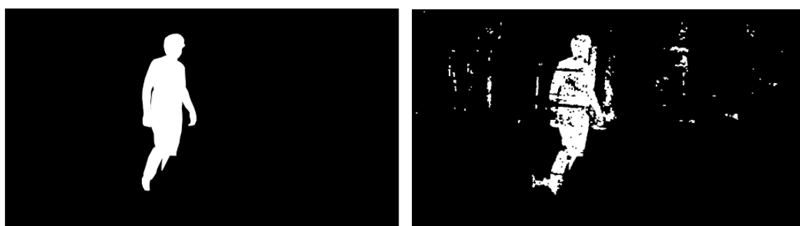
Frame 350 - Ground truth and extracted foreground
