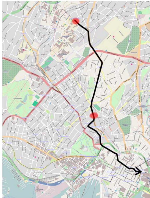
Figure 3.9: The tram route used to test the transparent handover solution. The two marked areas show where WLAN was available.
