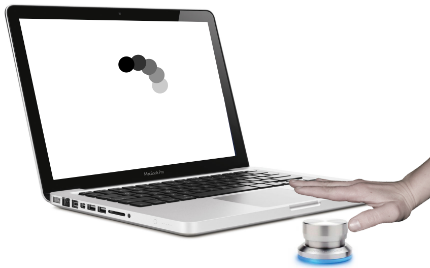
Figure 4.1: Experiment setup for investigating sensitivity to delay. The screen presents stimuli while the button receives input.
