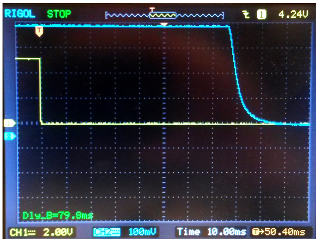
Figure 3: Capture of trigger event. Yellow line represent output from the mouse, blue line represents output from the photosensor. Both are active low. The difference in time between the two flanks are shown in green in the bottom-left corner of the oscilloscope screen.
