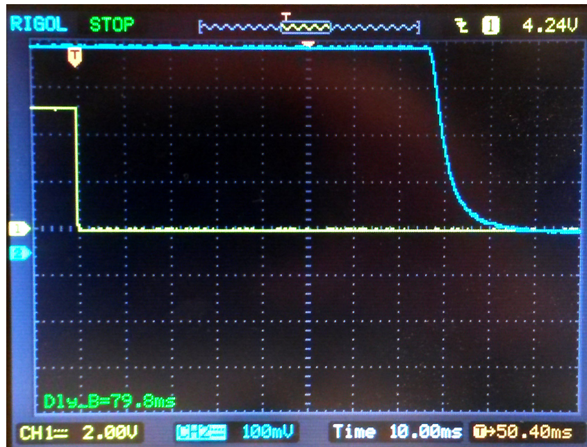
Figure 3.4: Capture of delayed event. Yellow line represent output from the mouse, blue line represents output from the light sensor. Both are active low. The difference in time between the two flanks is shown in green in the bottom-left corner of the oscilloscope screen.
