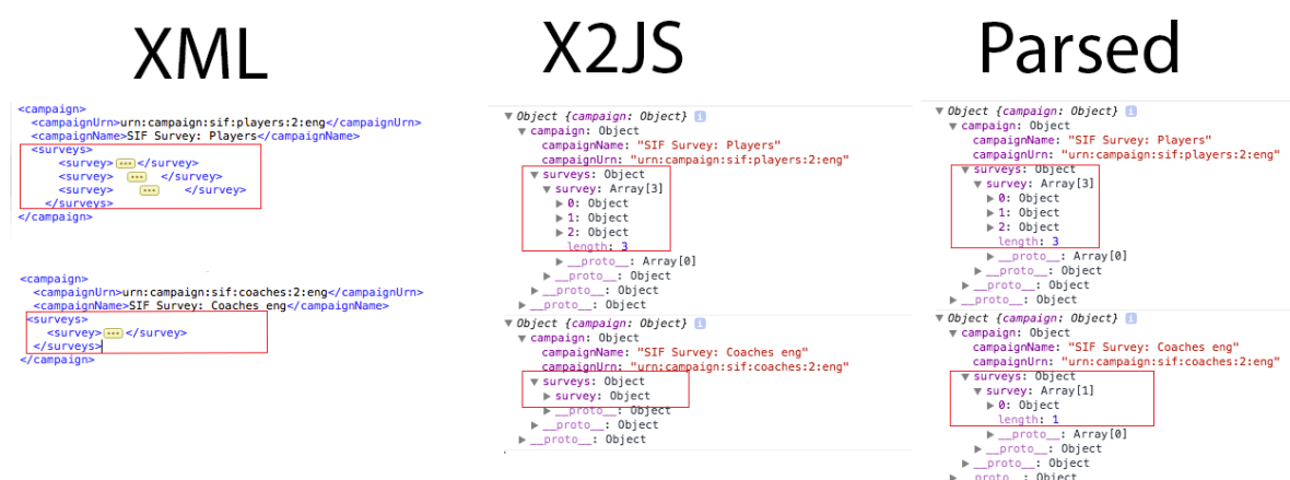
Figure 4.11: X2JS converting XML to JSON
