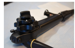
(d) The controll unit of the endo- scope the gastroenterologist uses to zoom, rotation, etc.
