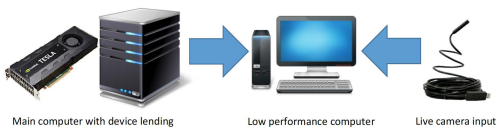
Figure 4: A complete overview of the demo setup. The demo consists of 2 computers, 1 Dolphin interconnect device, 1 screen, an artificial colon and a flexible camera. The users can use the camera in the flexible colon and will get real-time feedback about possible findings. Furthermore, the demo can be switched between Device Lending on and off to demonstrate the effect of it more clear.
