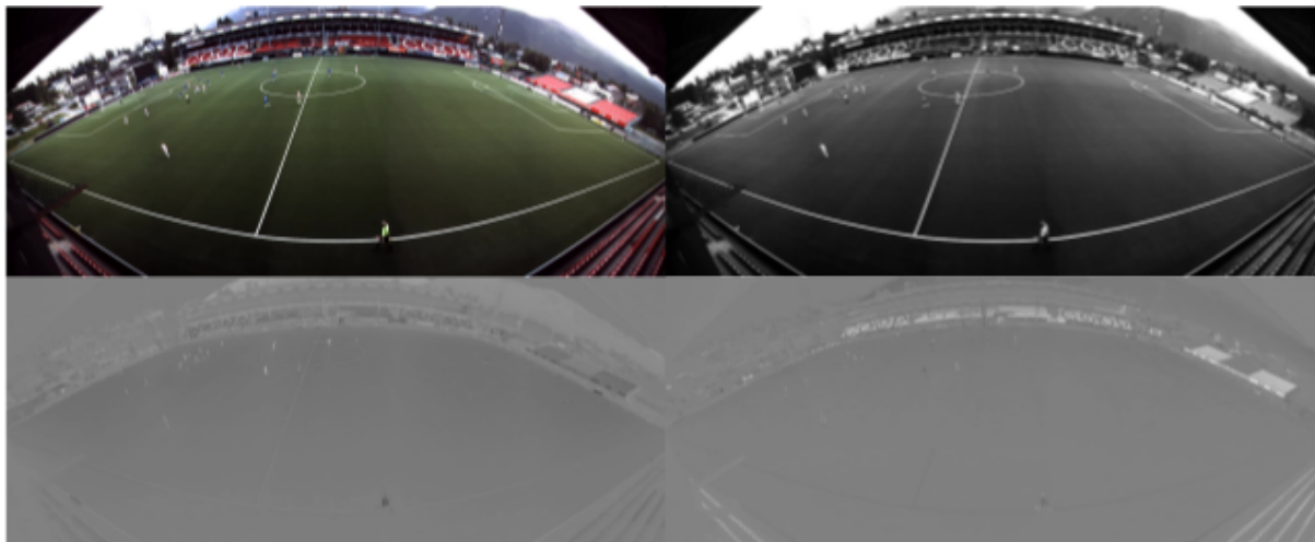
Figure 3.4: Illustration of YUV combined and each channel in YUV separated in greyscale
