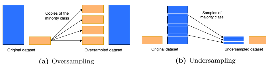
Figure 2.10: Two popular resampling methods. Oversampling (2.10a) make copies of the minority class until all classes have the same amount of samples, and undersampling (2.10b) sample from the majority class until it reaches the same amount of samples as the minority class.
