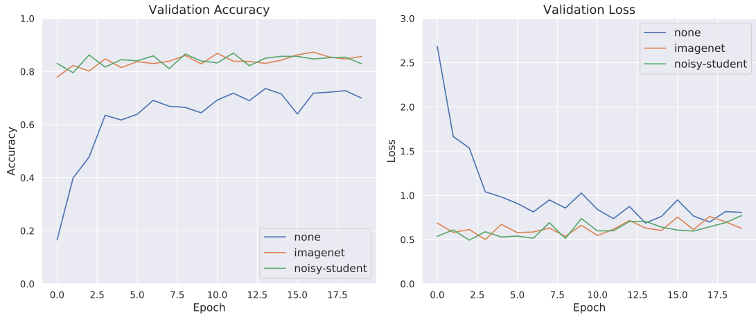
Figure 4.6: EfficientNetB0 trained for 20 epochs with different layer weights initialization. The data points are collected from measuring the model performance on the validation set during training. Blue line; no pretrained weights, red line; pretrained weights on ImageNet with AutoAugment, green line; pretrained weights from noisy-student.
