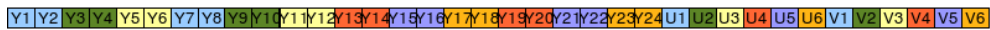
Figure 6.4: 4:2:0 YUV packed chroma subsampling. This is similar to H.264's 4:2:0 YCbCr with Cb and Cr represented as U and V. The figure is from Wikipedia's article on YUV [6] with modifications.
