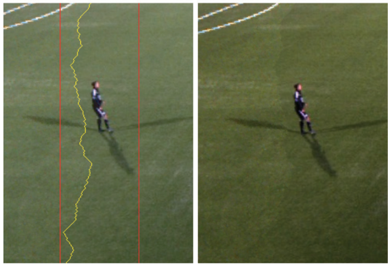
(c) Dynamic stitch with no color correction. In the left image, one can see the seam search area between the red lines, and the seam in yellow. In the right image, one clearly sees the seam going outside the player, but there are still color differences.
