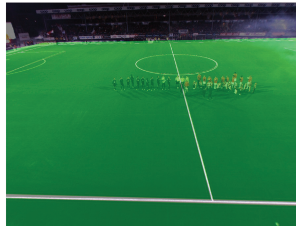
(d) Warping and superimposing the ZXY plane onto the image from camera 2.
