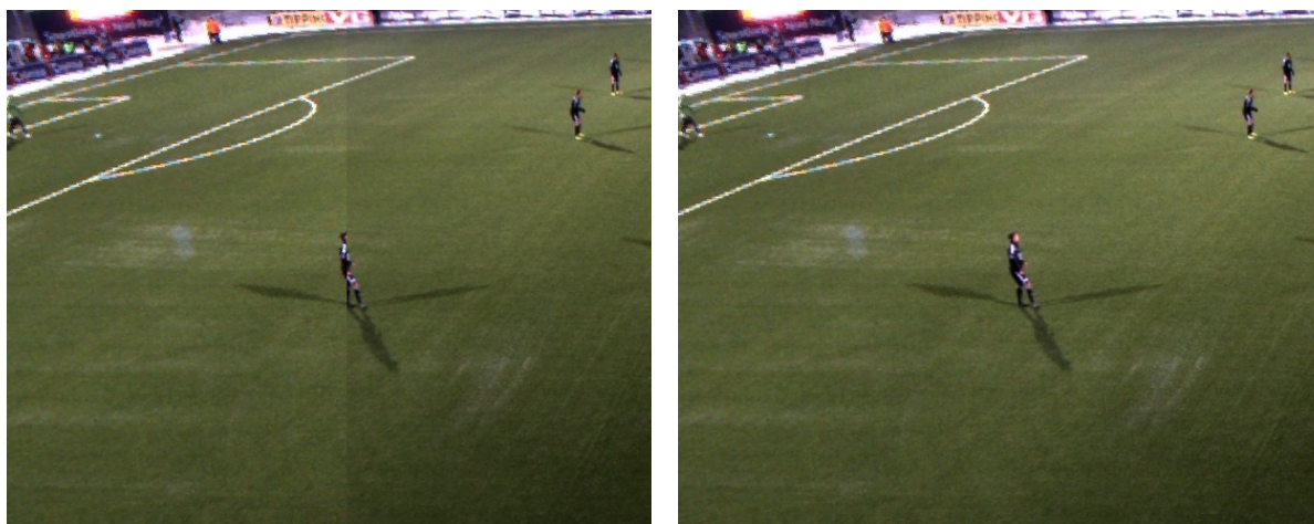
(a) The original fixed cut stitching with a straight vertical seam. (b) The new dynamic stitching with color correction.
