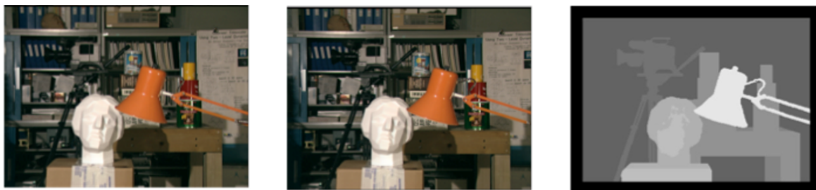
Figure 2.8: Illustration of depth estimation. Courtesy: Middlebury Stereo Vision Dataset 6
