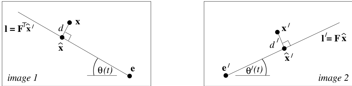
Figure 4.4: Illustration of epipolar geometry. Courtesy Multiview Geometry (Hartley and Zisserman, 2004)
