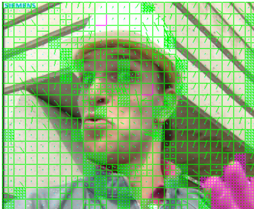
Figure 2.3: Motion vectors. Inter-coded macroblocks are displayed as green, intra-coded as purple. The line extending from the center of each green block corresponds to the motion vector.
