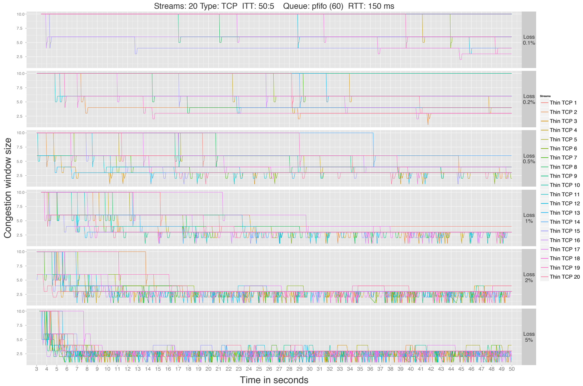
Figure 4.7: Congestion window growth for 20 thin streams with TCP Cubic using default kernel settings
