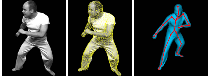
Figure 3.5: Original image (left) with the mesh (center) and skeleton (right) next to it. Image taken from [19].
