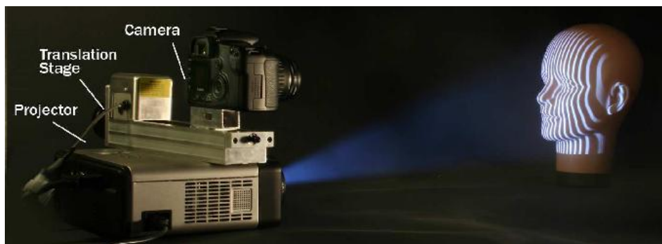
Figure 4.6: Vision-based gesture recognition can be achieved by a structured light approach. With structured light the depth information is obtained by projecting a pattern of structured light, and look at the way this pattern deforms when hitting a surface (such as the doll's face in the picture). Picture from Ramamoorthi (2007)
