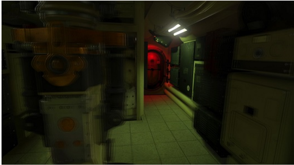
Figure 3.3: Positional jitter can make objects near the user seem "blurry" or unfocused. In the image the objects near the user are more blurry than those that are farther away. This is because these object "move" more, relative to the user, from frame to frame as the user's head moves. Picture from Antonov (2015)
