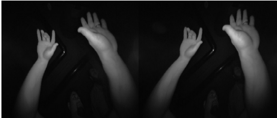
Figure 4.5: Stereo image captured by a stereoscopic vision device. These images are compared by looking at differences (offsets) in the object's position and create a disparity image which is used to obtain depth information. Picture from Colgan (2016)
