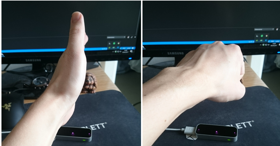
Figure 5.3: The palm-side gesture (left) is used to move the user left and right along the x -axis. The fist gesture (right) is used to move the user forward and backward along the z -axis.
