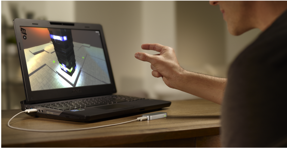
Figure 6.1: The Leap Motion Controller is a vision-based gesture recognition devices that can be placed on a table top to observe the users hands.
