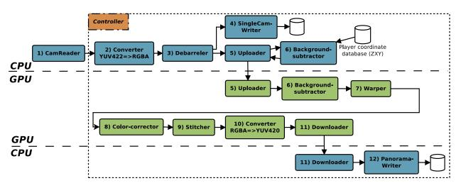
Fig. 5: The parallel and distributed processing implementation of the stitching pipeline.
