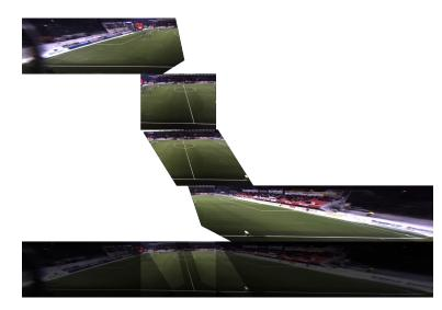
Fig. 3: The stitching process. Each image from the 4 different frames are warped and combined into a panorama.
