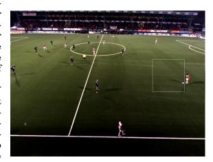
Fig. 15: An example of when the tracking box fails to capture the tracked player. Even though our analysis of the system indicate very infrequent errors, it may be various reasons for failed tracking, e.g., both clock skew, sensor system accuracy and coordinate mapping.
