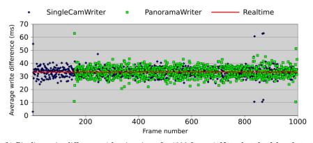
(b) Pipeline write differences (showing times for 1000 frames). Note that the delayed start of panorama writes is caused by the frame delay buffer implemented in the uploader module.
