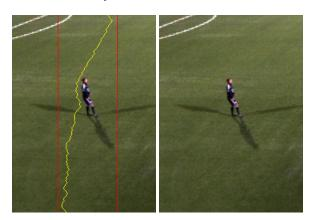
(d) Dynamic stitch **with** color correction. In the left image, one can see the seam search area between the red lines, and the seam in yellow. In the right image, one cannot see the seam, and there are no color differences.
