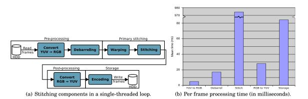
Fig. 4: The Bagadus single-threaded processing loop stitching implementation.
