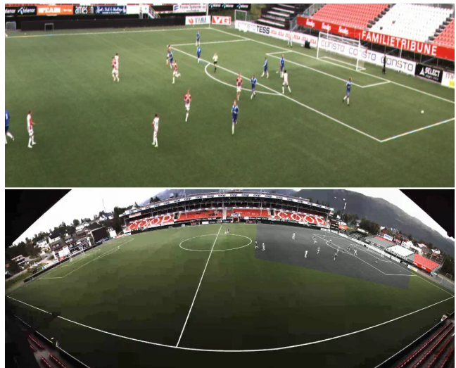
Figure 5: An example of a multi quality tiled-panorama and the virtual view that is extracted from it. The quality of the panorama is quite poor in the areas that are not being shown to the user. However if the user decides to pan quickly, she still gets a reliable low quality video instead of a black patch.
