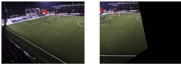
(a) Debarreled left image. (b) Warped left image.
