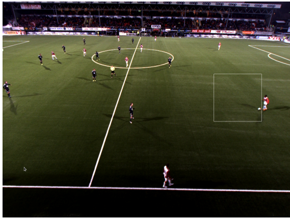
Figure 10: An example of when the tracking box fails to capture the tracked player. Even though our analysis of the system indicate very infrequent errors, it may be various reasons for failed tracking, e.g., both clock skew, sensor system accuracy and coordinate mapping.
