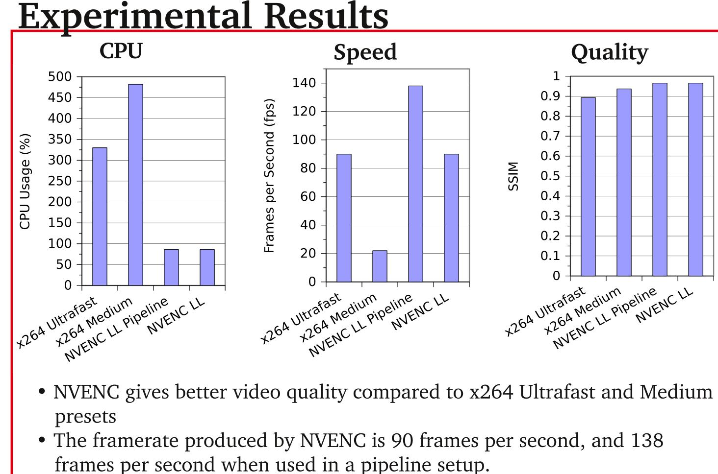
Experimental results from encoding 690 frames of the "tractor" 1080p test sequence with an Intel Core i7-2600 and NVENC on a NVIDIA Quadro K2000 GPU
